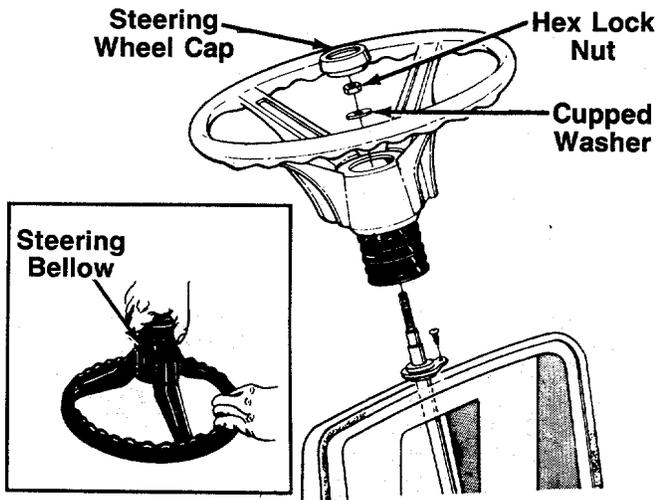
3. Attach one end of steering bellow to the steering wheel as shown in figure 6, inset.
