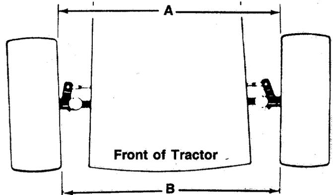
FIGURE 15. TOE-IN DIAGRAM
